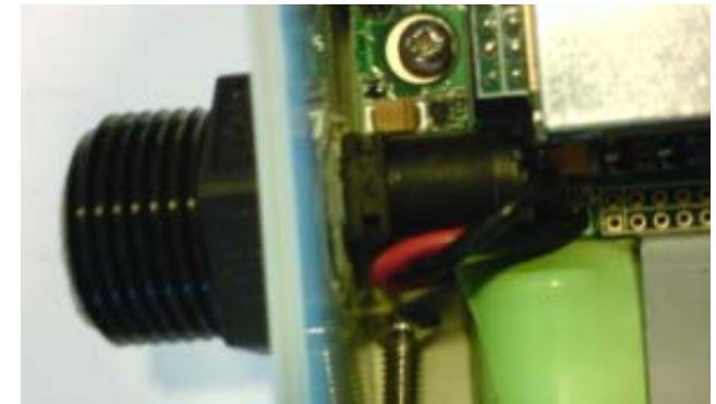
Figure 1-4 DC Gland and Power Connector
